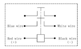
Note: The coil has polarity, The load and Aux. have no polarity
