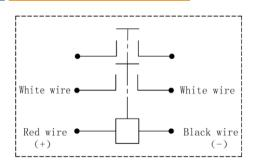
Note: The coil has polarity, The load and Aux. have no polarity
