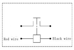
Note: The coil and the load have no polarity
