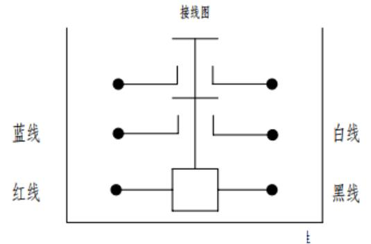
Note: The coil has no polarity, The load and Aux. have no polarity
