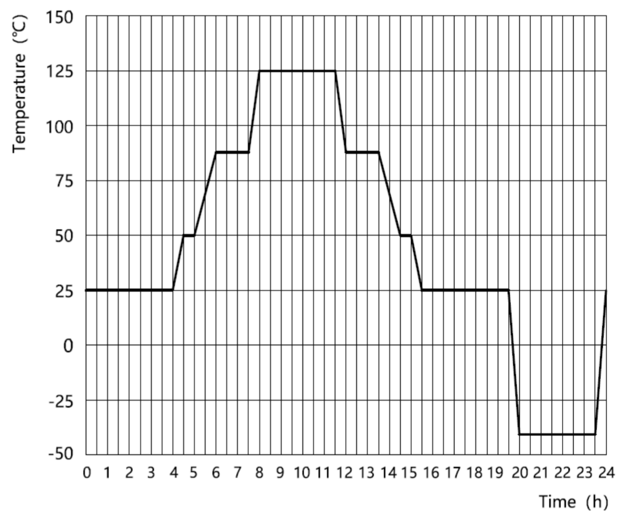
Ambient Temperature Curve of the Electrical Endurance Test
